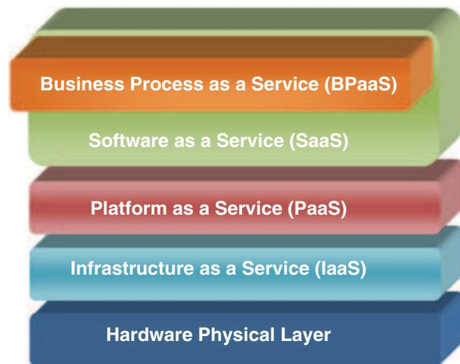
**Fig. 9.2** The Cloud stack extended by business process as a service (BPaaS)
