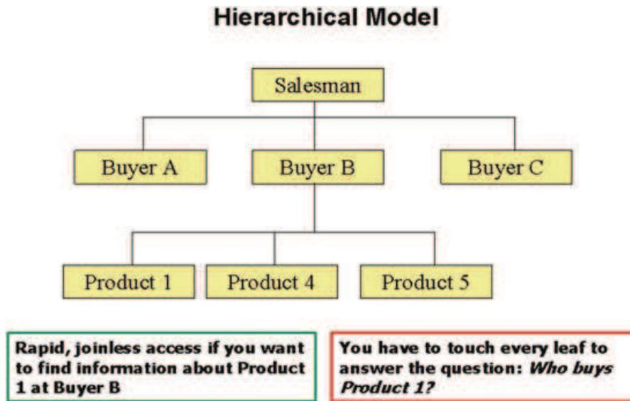
**Fig. 6.1** The hierarchical data storage model
